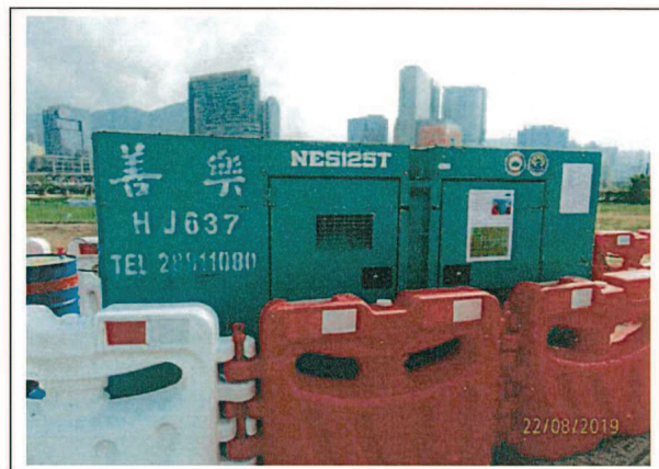
Generator, with Quality Powered Mechanical Equipment Label showing a Sound Power Level \leq 93 dB(A)
